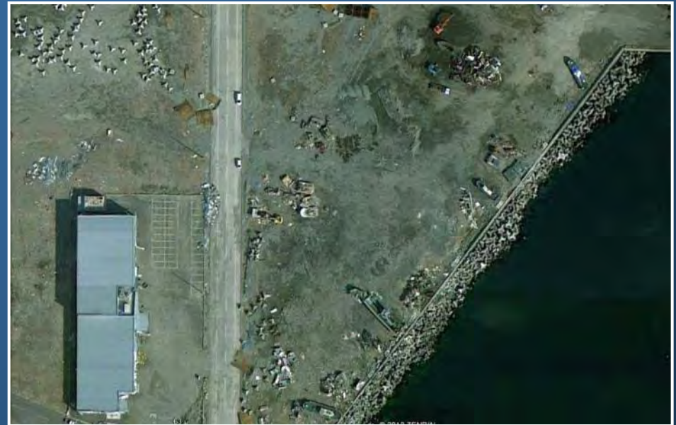
IX ITIS 2012 : Ripraps are detached and/or moved
